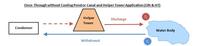
Withdrawal: Report the water that is removed from a water body for cooling, i.e. water used through the condenser.
